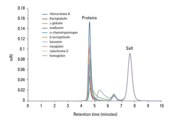
Proteins in 0.1mol/L phosphate buffer, pH 6.7 Mobile phase: 0.01mol/L KH<sub>2</sub>PO<sub>4</sub>/Na<sub>2</sub>HPO<sub>4</sub>, pH 6.7, 0.01mol/L Na<sub>2</sub>SO<sub>4</sub> + 0.05% NaN<sub>3</sub>
