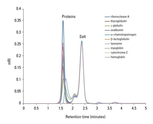
Proteins in 0.1mol/L phosphate buffer, pH 6.7 Mobile phase: 0.01mol/L KH<sub>2</sub>PO<sub>4</sub>/Na<sub>2</sub>HPO<sub>4</sub>, pH 6.7, 0.01mol/L Na<sub>2</sub>SO<sub>4</sub> + 0.05% NaN<sub>3</sub>
