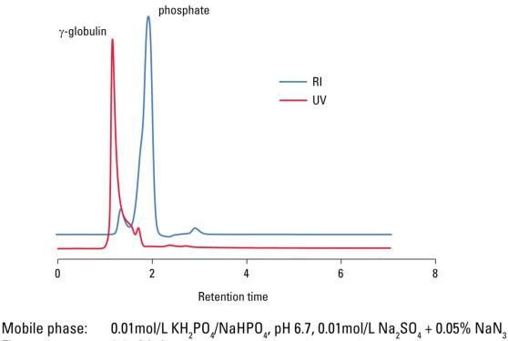
Mobile phase: 0.01mol/L KH<sub>2</sub>PO<sub>4</sub>/NaHPO<sub>4</sub>, pH 6.7, 0.01mol/L Na<sub>2</sub>SO<sub>4</sub> + 0.05% NaN<sub>3</sub> Flow rate: 0.8mL/min. Detection: UV@280nm and RI Temperature: ambient
